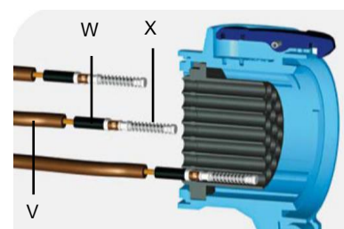
V : isolated conductor W : isolation sleeve on ferrule X : socket-outlet contact
